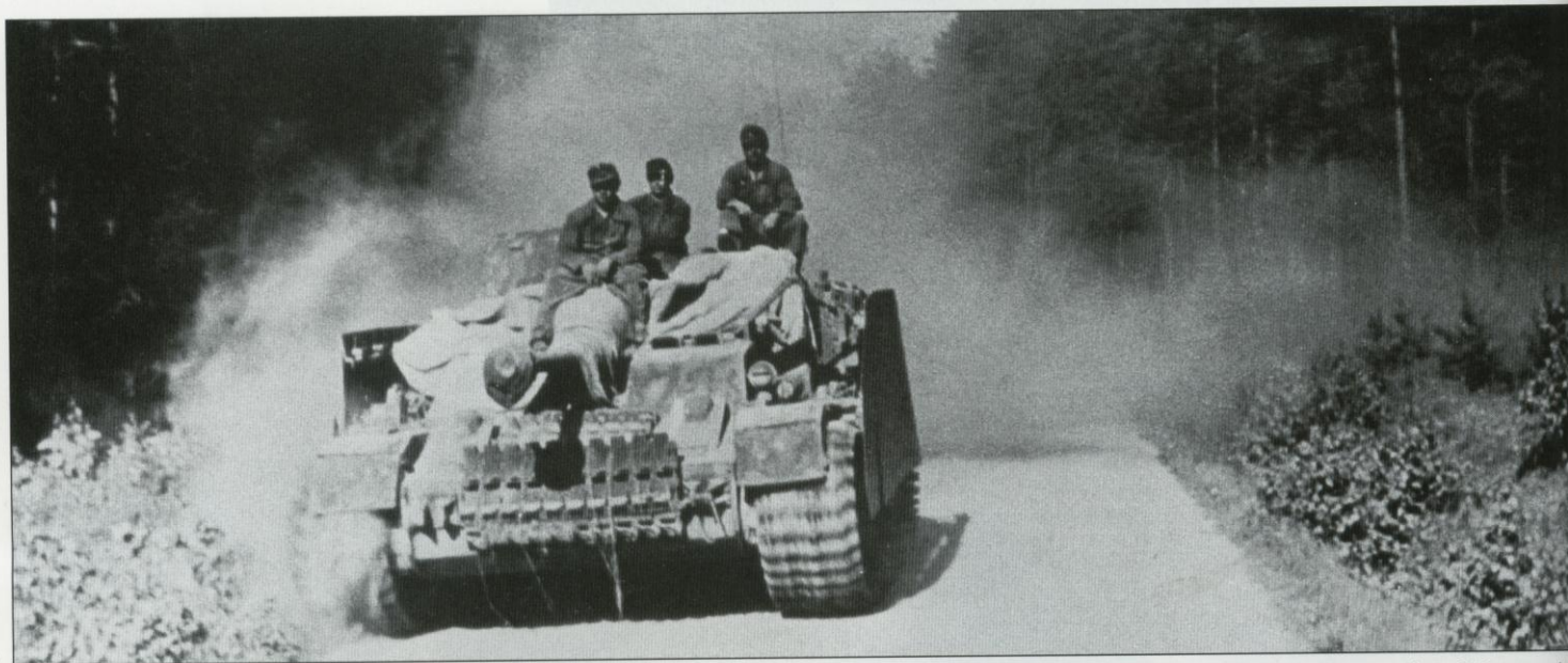
A StuG IV kicks up a cloud of dust as it advances down a forest road. Note the interesting camouflage pattern (most probably green) and the special wider tracks. These tracks were developed in 1944 based on the experience acquired through the use of "Ostketten" in the two previous winters. It is possible that their use was widespread in divisions fighting on the Eastern Front, even though they appear in only a few photos.
