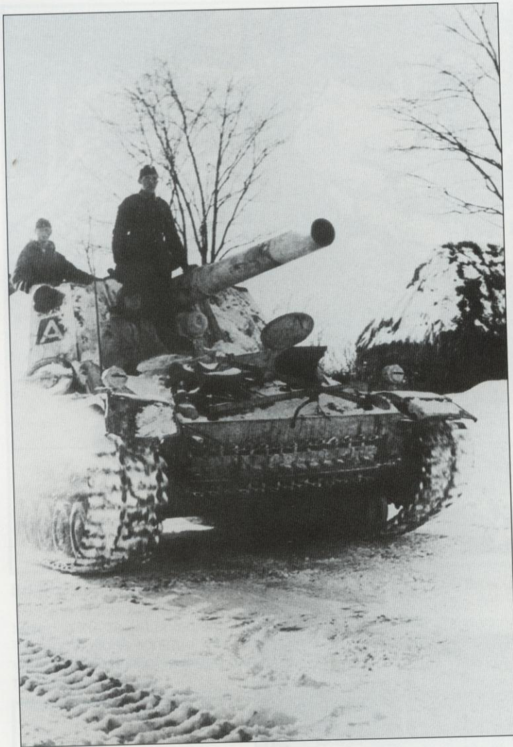
This series of three photos provides a view of a maneuvering battery of Hummel 15cm self-propelled howitzers belonging to an independent battalion of heavy artillery. All three vehicles (marked with the letters "A", "G", and "O") are equipped with wide "Ostketten" and are partly or completely camouflaged with white paint and snow.
