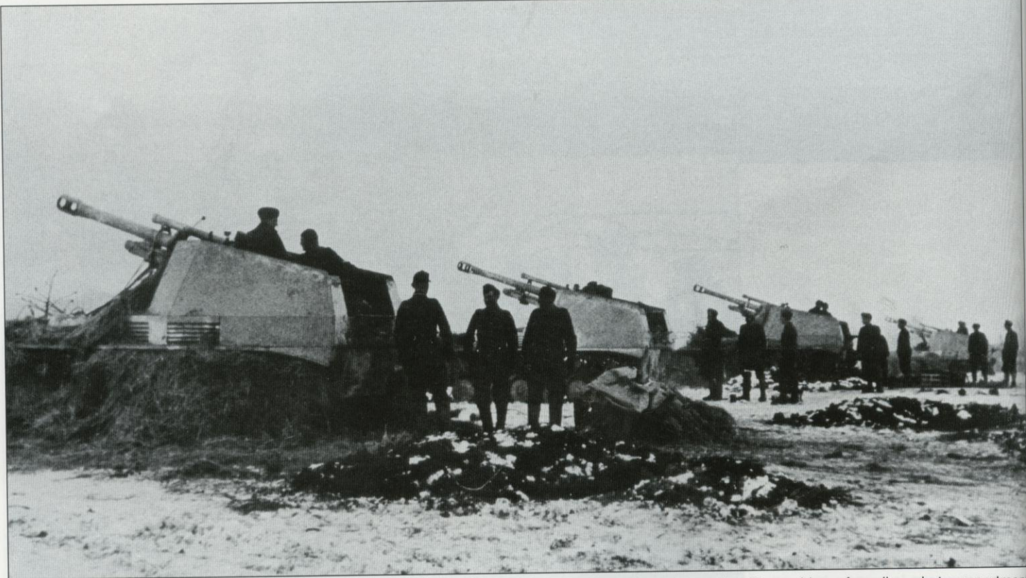
A battery equipped with Wespe (wasp) 10.5cm light self-propelled field howitzers stands ready to open fire. The problem of small combat compartment was even greater with the Wespe than with the Hummel. As we can see in this photo, three out of five crew members must perform their duty outside the vehicle. However, the Wespe could carry twice as many shells as the Hummel.
