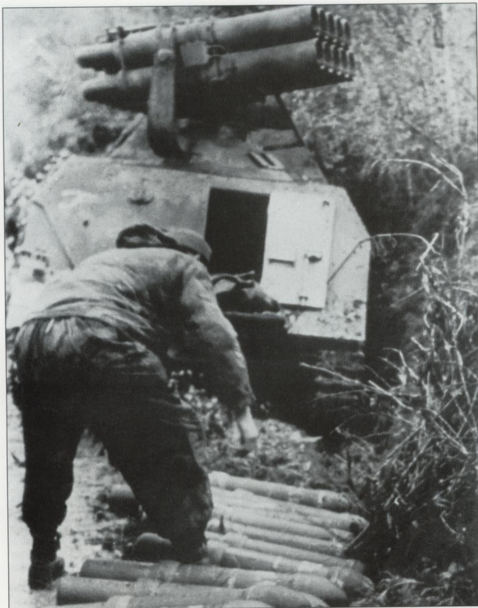
This photo shows over a dozen 15cm rockets ready for loading into the Panzerwerfer 42. The lightweight 10-kg (22-lb) warheads were installed in the rear of the missiles and when they exploded they had a terrible impact on any living target within a 13 x 40-meter (14 x 44-yard) area.
