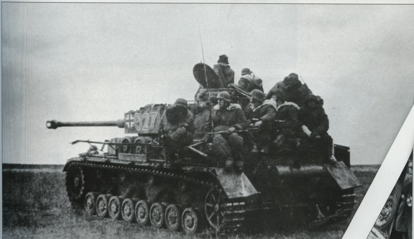
A Pz.Kpfw. IV Ausf. H transports a squad of infantry during the fighting in the autumn of 1943. It is interesting to note that the soldiers are wearing reversible parkas to protect the hull. Those installed on the left side were lost, probably as a result of combat. The soldiers wear reversible parkas, normally gray and white, but this photo shows that the parkas of two of the soldiers have dark (black?) interiors.
