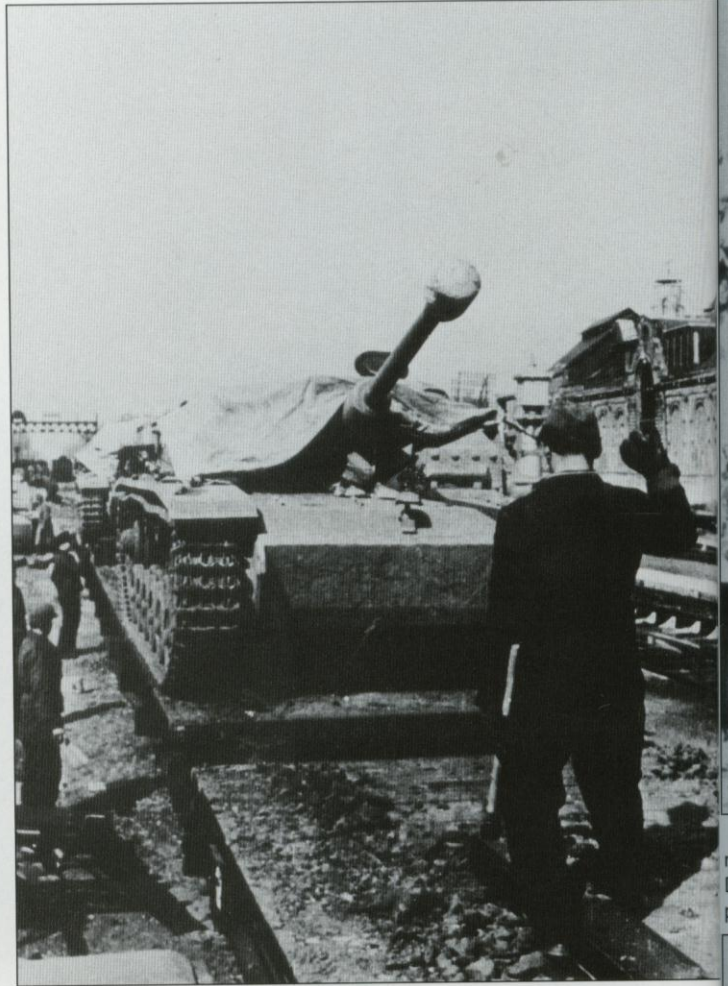
StuGs are loaded onto a flatbed railroad car for shipment to the front lines. The photo shows that the vehicles were transported from the manufacturer without side skirts, which were usually installed in divisional workshops.
