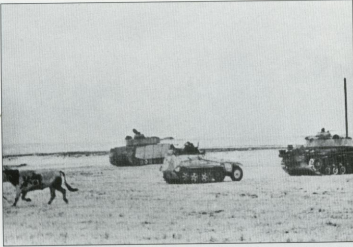
Three different vehicles belonging to a staff unit from a tank battalion roll across the frozen winter landscape. At right is the Pz.Bef.Wg. III Ausf. K, in the middle is a command model of the Sd.Kfz. 250, and in the background is a Pz.Kpfw. IV. All the vehicles are painted in winter camouflage (the bull's winter coloring is natural).
