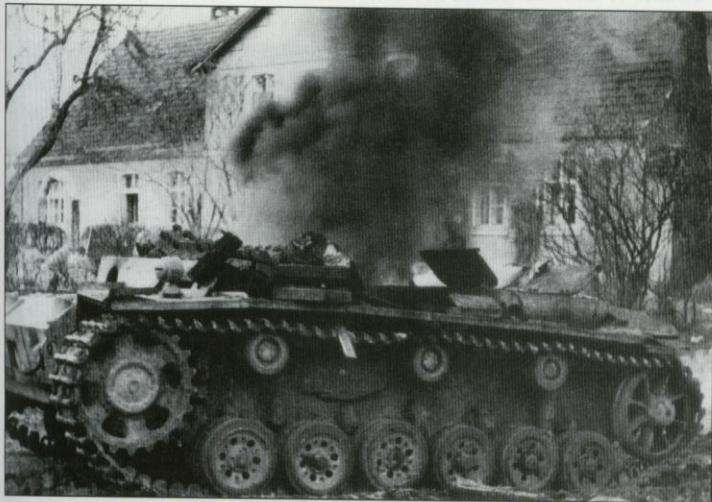
A recovery tank, known as the Bergepanzer III, burns in a German village somewhere in Pomerania in March 1945. This vehicle was converted from a Pz.Kpfw. III that was returned for overhaul in 1944. They were issued to the workshop companies of Panzer units equipped with StuG III's and IV's. The tank has additional front armor on the superstructure but is lacking a machine gun.
