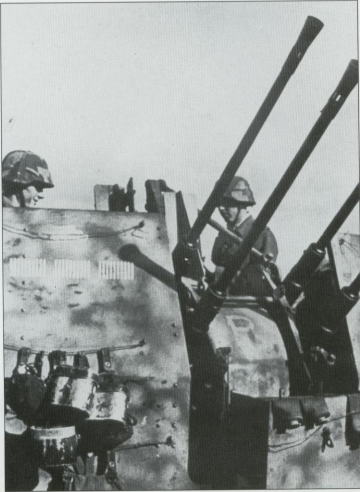
Another very successful anti-aircraft weapon: the 2cm Flakvierling 38 gun, which was usually installed on half-tracks. It is decorated with 30 victory markings, which indicate that the crew scored that many victories over enemy aircraft, and the silhouette of tank that fell victim of the anti-tank shells fired from the gun. The letter "P" is visible between the barrels.
