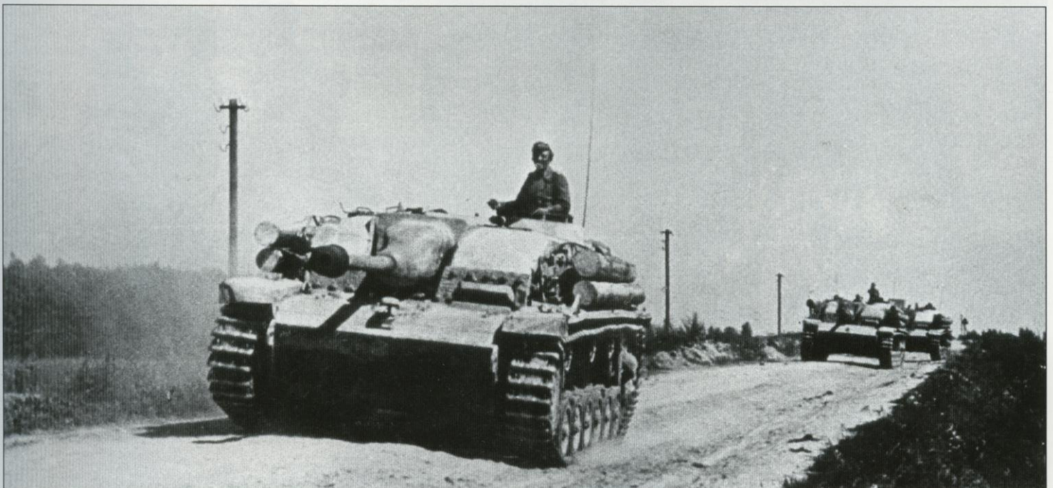
A platoon of late production StuG III Ausf. Gs passes in review for the camera along a dusty road. All the vehicles lack their side skirts, but large wooden logs have been mounted for protection instead. The lead vehicle is fitted with the late-style "Saukopf" mantlet.
