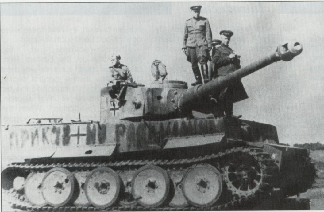
The aftermath of the Battle of Kursk, where heavy losses were inflicted on both the German and Soviet armies. This Pz.Kpfw. VI Tiger I, which was a unit commander's vehicle, was damaged by the Soviets and abandoned by its crew. Note the Cyrillic inscription on the side of the superstructure and the penetration holes. The tank was captured by the Soviets on 10th August 1943 near Grajvoron.
