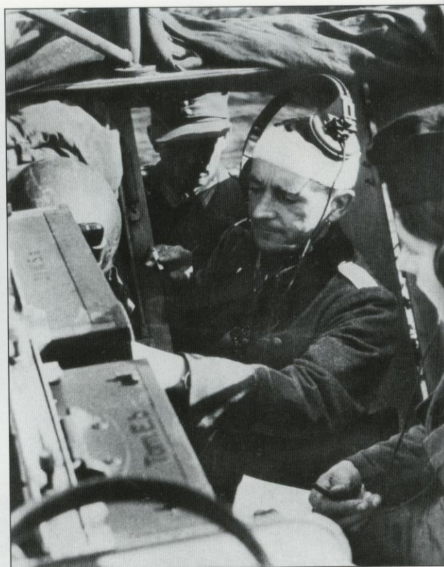
Here we see radio operators at work in the combat compartment of the Sd.Kfz. 250 Neu half-track. Many of these vehicles carried the famous "Enigma" radio sets that assisted the higher level German staffs to control the operation of the war. Note that this ground-to-air communications vehicle has a very cramped interior. The Sd.Kfz. 250/3 Neu carried a rod-and-star aerial instead of the frame aerial.
