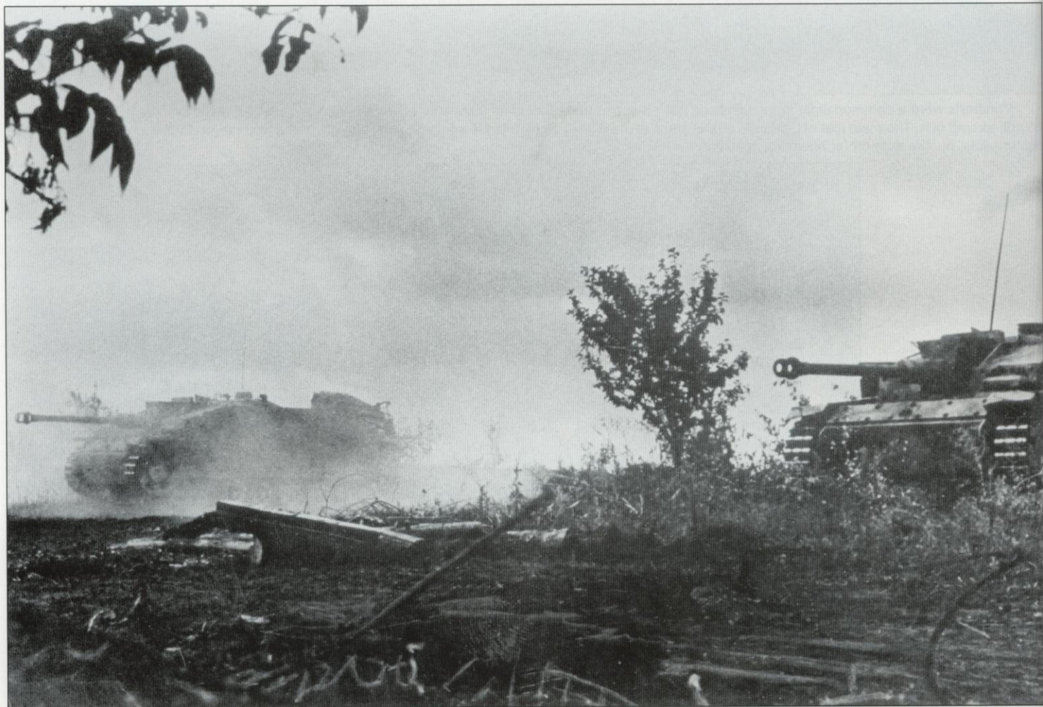
Another shot of Ausf. Fs in a similar situation. Note that both vehicles are equipped with side skirts with additional armor on the frontal plates of the hull and superstructure. Both modifications, which were originally designed for the Ausf. G model, indicate that these vehicles were modernized in the factory during overhauls.
