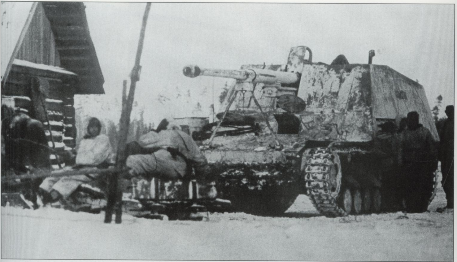
The "brother" of the Hummel was the Nashorn tank destroyer. This SPG, which was armed with an 8.8cm Pak 43/1 (L/71) gun, was the best destroyer of armored targets on the Eastern Front in the second half of the war. It was light, mobile and very powerful. The AT shell fired from this gun could destroy any tank used by the Red Army — including the heavy IS-2 — at a range of 2,000 meters (2,186 yards).
