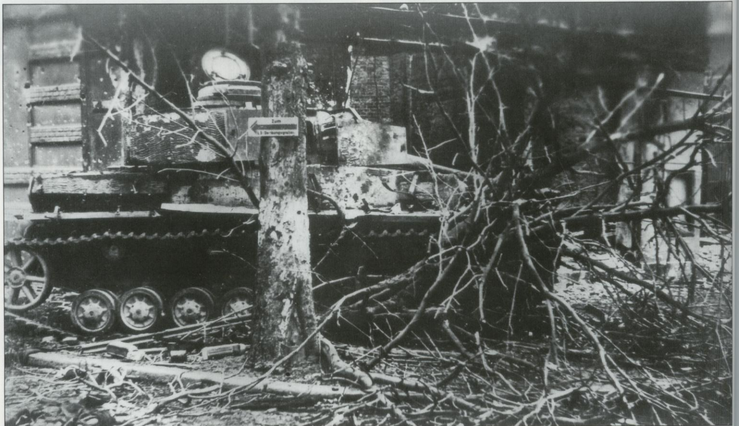
This profile view of the remains of a destroyed Pz.Kpfw. IV photographed in Pomerania in the spring of 1945 shows the resulting fire damage on the exterior of the tank. Note the pattern in which the Zimmerit anti-mine paste was applied to the turret skirting.
