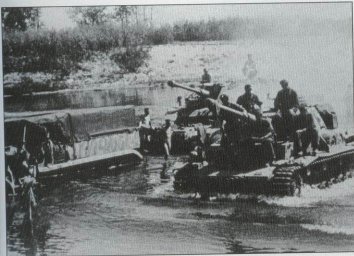
Photographed in September 1943, vehicles belonging to an armored division cross a river. At the left is a Sd.Kfz. 7 tractor, at the right a Pz.Kpfw. IV Ausf. G is visible, and in the background is a StuG III. All vehicles are painted in the three-color (dark yellow, olive green, red brown) camouflage scheme introduced in the spring of 1943.
