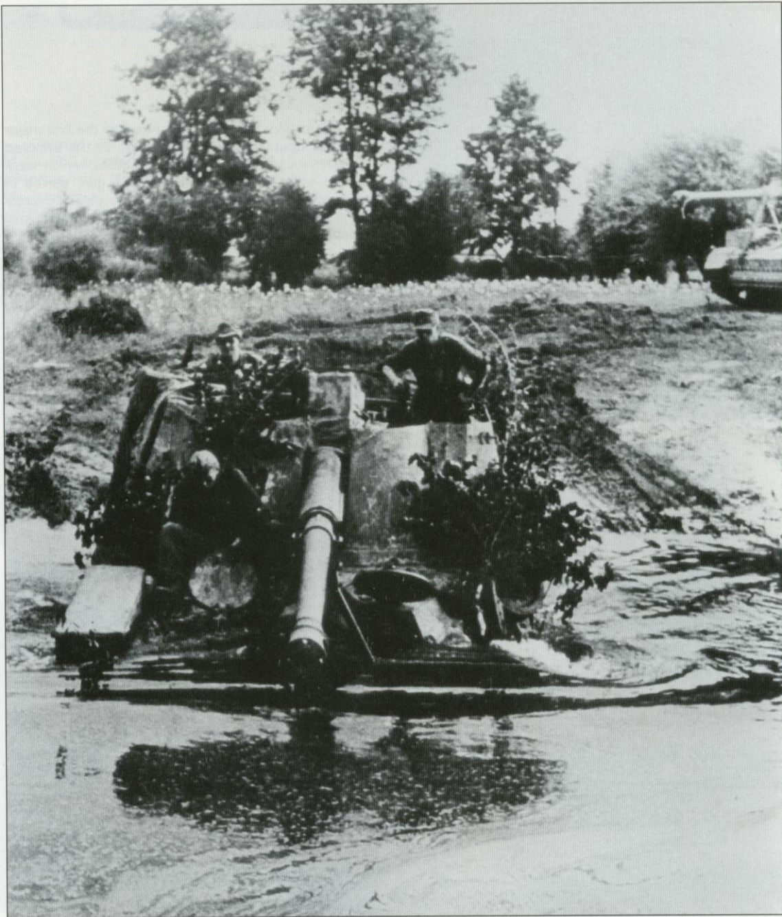
The most feared Panzerjäger (tank hunter) was surely the Nashorn. Armed with the mighty 8.8cm PAK 43/41, these self-propelled guns decimated Soviet tank formations from distances of over 3,000 m (3,028 yards). These vehicles are seen here crossing a narrow ford. Both are finished in plain dark yellow.
