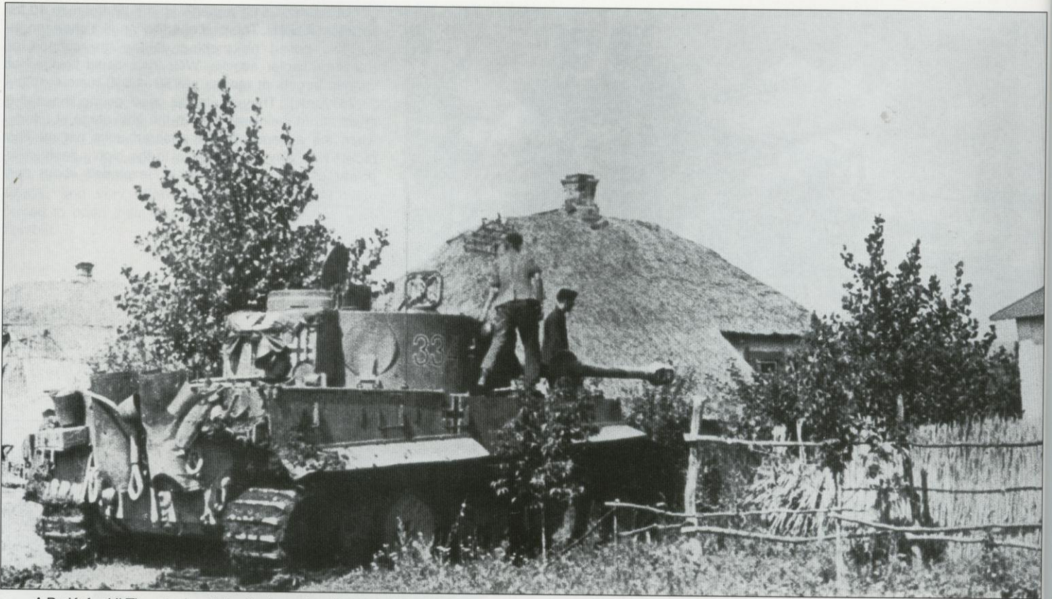
A Pz.Kpfw. VI Tiger tank with tactical number "334" and national crosses painted on all sides of the turret. The tank carries a Nazi flag for air identification, smoke candle dischargers, and is most probably camouflaged with small olive green spots on the superstructure and a bigger pattern in the same color on the turret.
