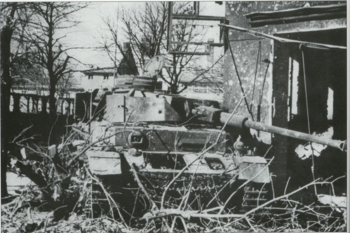
Looking just as decrepit as the buildings and landscape that surround it, a Pz.Kpfw. IV sits abandoned in Pomerania after being destroyed during the fighting there in the spring of 1945. Note the conspicuous absence of the bow MG34 in the ball mount.
