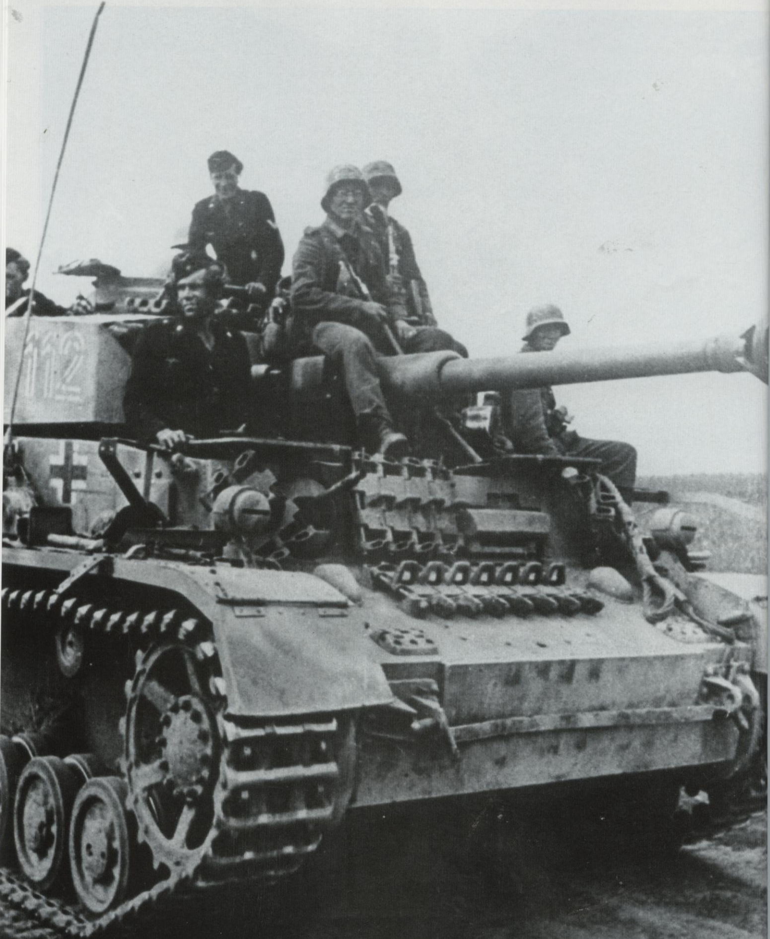
A late production Pz.Kpfw. IV Ausf. G gives a few troopers a lift. Additional armor was welded to the front of the hull. Note the turret spaced armor attachment points for armored skirt on the right side of the tank. Usually only turret skirts were installed; tank crewmen preferred their use over the full set of skirts. Also note that the tactical number is painted only with a white outline in the manner that was typical from the autumn of 1943.
