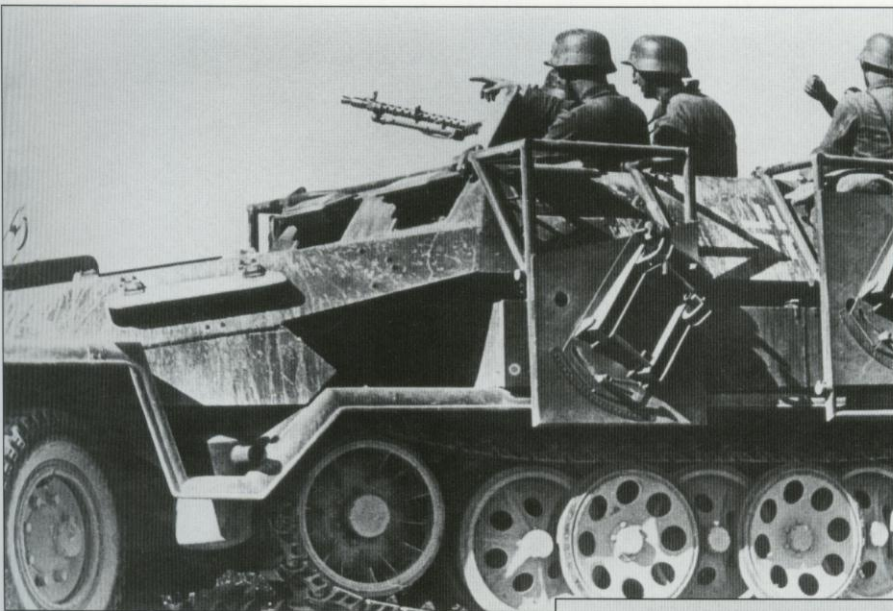
A Sd.Kfz. 251/1 armed with the Wurfrahmen 40 for six 28cm rockets. This sort of artillery had a short range, but this posed no problem during the support of Panzergrenadier attacks. WGr 280s could be fired at various targets at ranges of 750 -1,900 meters (820 - 2,078 yards). They could be used during the entire attack, from their own lines to the final stage of attack, when the advance of the armored units began. The rocket was very effective due to the highly destructive power of the warheads, which exploded about one meter above the ground.
