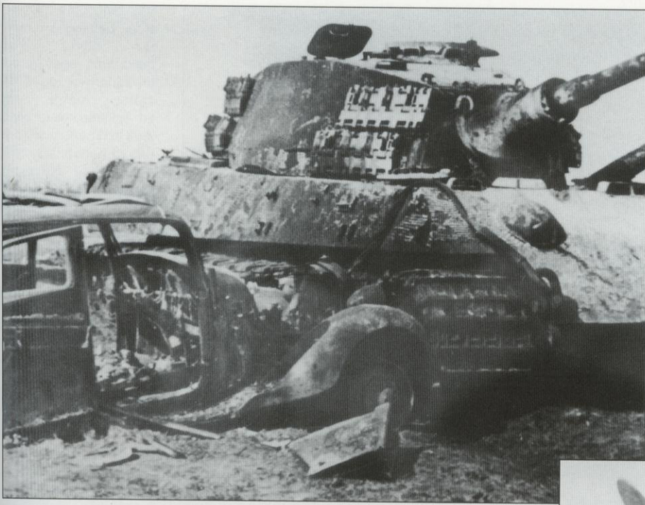
The end of a Tiger. This burned out Tiger II Ausf. B, with Henschel Production Turret, sits on a beach on the Frisches Haff in April 1945. The 8.8cm KwK 43 L/71 gun was probably the best tank weapon in WWII, being able to knock off its opponents with ease. However, the Tiger II entered service too late to change the outcome of the armored war.
