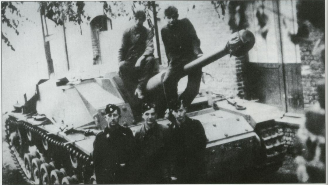
The crew of this StuG III Ausf. G is seen taking a group picture. The bolt-on armor to the superstructure and the hull front is evident.
