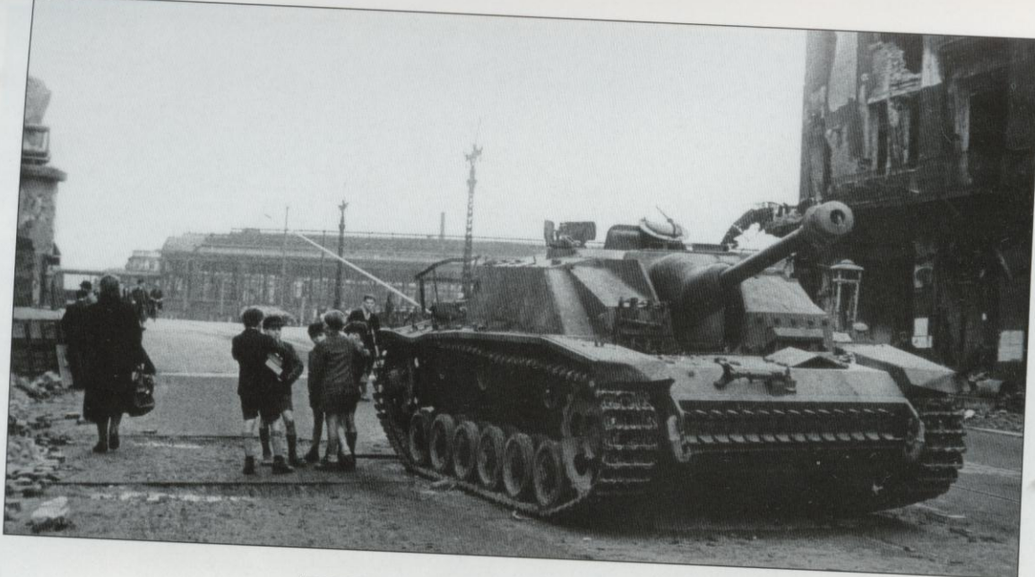
This StuG III Ausf. G was abandoned in the middle of a Berlin street in May 1945. The vehicle is equipped with the "Saukopf" mantlet and the "Saukopf" remote-control machine gun with the small armored shield. During the last two weeks of fighting in the Berlin area, the Germans lost about 850 tanks and self-propelled guns, many of them being abandoned due to breakdowns or lack of fuel. The Soviets claimed that they destroyed over 1,700 enemy tanks, however.
