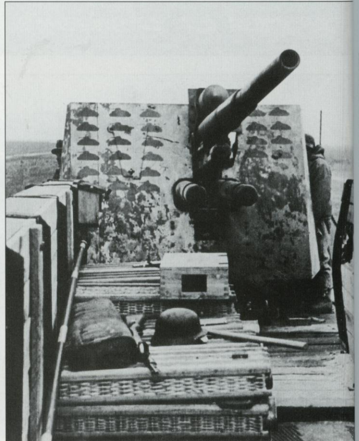
Another "88" gun from the same Eisenbahnpanzerzüge displays its successes: 26 tank "kills" on the gun shield and seven or eight air victories on the barrel. Note the damage to the right "armor plate" (composed of sand in a wooden framework), and that the gun has a dark gray barrel and a sand-colored shield.
